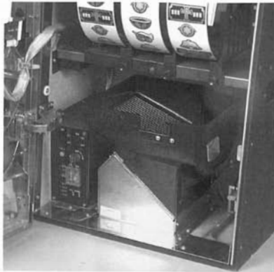
Figure 2: Hopper properly seated in its tracks
